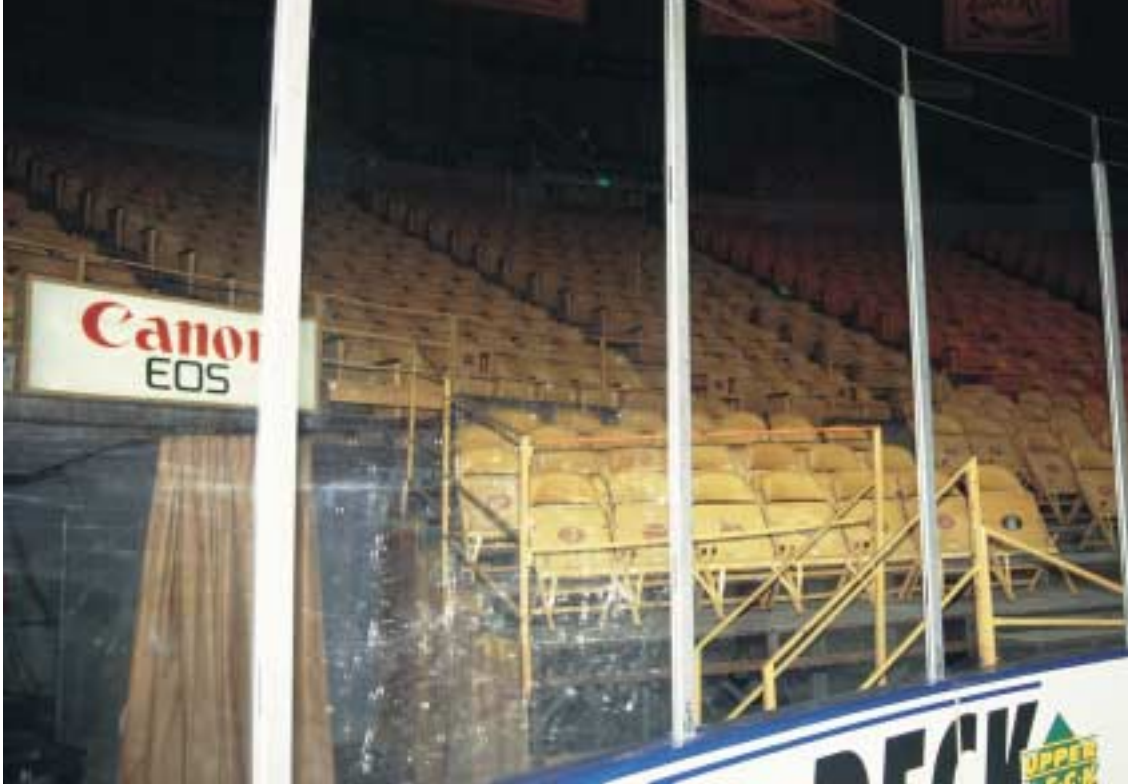
The ACRYLITE GAR acrylic sheet panels on the right side still allow for a clear view. Meanwhile, the two uncoated sheet panels on the left have become scuffed and marred.
